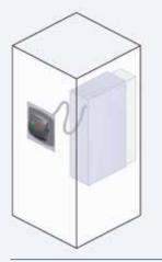
Remote installation on exterior of enclosure
