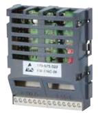
The EM-ENC-04 speed sensor module extends the standard terminal board of the inverter, providing an interface for line driver speed sensors with Z channel. This module is able to manage TTL, HTL, or push-pull incremental speed sensors to standard EIA RS422 (line driver). The EM-ENC-04 speed encoder module is equipped with 6 control terminals for A,  $\overline{A}$ , B,  $\overline{B}$  direction signals and Z and  $\overline{Z}$  zero signals transmitted by the speed sensor.
