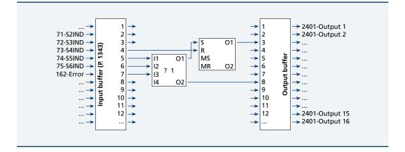
Sophisticated control routines design is within range with new logic functions. Software developers will be able to adjust drive controls fitting automation requirements, simply combining the 16 inputs with the 32 function blocks available and achieving results in the 16 output latches. Following features are implemented:
