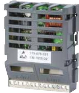
EM-RES-02 angular position transducer module extends the standard functions of the frequency inverter by providing a supplementary input for a resolver. This module shares all the features of EM-RES-01 except for the emulation of the encoder zero signal, which in this case replaces the Systembus port.
